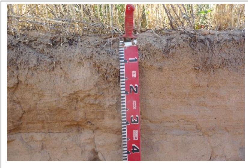
Figure 4 Topsoil of site P03B showing the effects of standard cultivation (control treatment).
